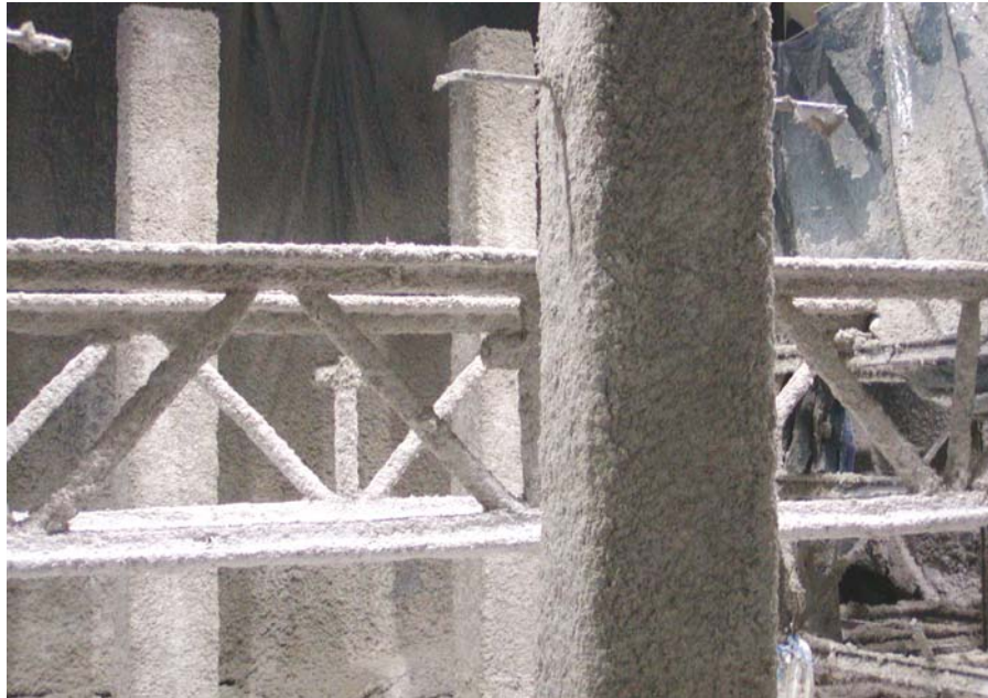
Figure 6-42. SFRM-coated steel components prior to a test.
